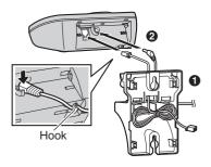
3 Insert the hooks on the wall mounting adaptor into the holes **A** and **3** on the base unit.
